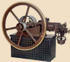
Original Otto Four-Stroke Engine, 1895 World's first combustion engine, by Nicolaus August Otto, which motorized the world from Cologne. – Power 1 HP at 250 rpm. Fuel: Petrol. Weight: 490 kg. Size: 69 x 24 x 58 in. – Perfect working condition! – Estimate: Euro 20,000 – 30,000 / US$ 25,000 – 40,000
